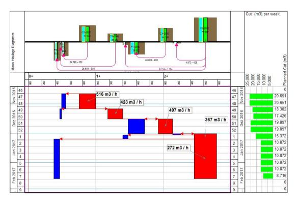
Although the same resources are used in each task, the production rate differs based on the transport distance. The bigger the distance, the lower gets the production rate.
