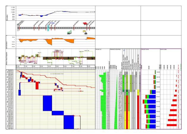
Scheduling mass haulage operations is easier and can be done in faster and and more accurately. Filter the Mass Haulage Diagram by haulage type, select the haulages and use the wizard to create the cut and fill tasks. Resources get assigned based on the templates for that specific haul type. The wizard links the series of cut tasks created by finish to start links. If the cut task is adjusted, the fill task duration is automatically updated.
